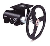
El-O-Matic MO series declutchable gear operators offer simple and reliable manual positioning of the valves, dampers and other quarter turn devices when overriding existing pneumatic or hydraulic rotary actuators. All El-O-Matic MO units combine rugged construction, light weight and modular design to provide the most efficient and cost effective solution to a full range of manual override requirements.
